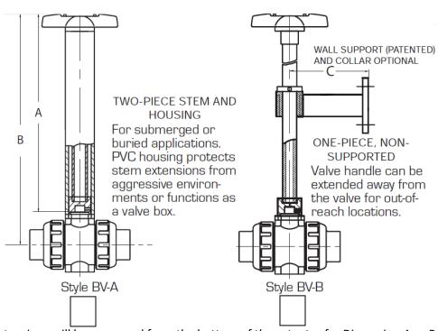
All actuator extensions will be measured from the bottom of the actuator for Dimension A or B.
