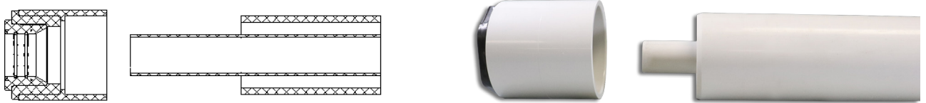
Figure 5: End termination and pipe after completion of step 1
