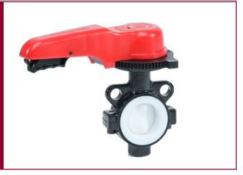
The Type-55 IS butterfly valve is well suited for a wide variety of applications. The Type-55 IS butterfly valve conforms to ISO 5752 Short Pattern face to face dimensions. This allows the Type-55 IS to directly replace metal valves conforming to the same standard. Available as ANSI B16.5 Wafer or ANSI B16.5 Lug models with 316SS drop-in lug inserts. Can be pneumatically or electrically actuated.
