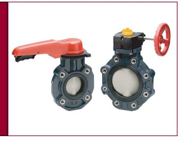
The Type-57 LIS butterfly valve is well suited for a wide variety of applications. The Type-57 LIS butterfly valve conforms to ISO 5752 Short Pattern face to face dimensions. This allows the Type-57 LIS to directly replace metal valves conforming to the same standard. Available as ANSI B16.5 Wafer or ANSI B16.5 Lug models with 316SS drop-in lug inserts. Can be pneumatically or electrically actuated.
