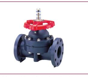
The Type-14 flanged diaphragm valve is well suited for a wide variety of applications. The Type-14 flanged diaphragm valve conforms to ISO 5752 Short Pattern face to face dimensions. This allows the Type-14 diaphragm valve to directly replace metal valves conforming to the same standard. Can be pneumatically or electrically actuated.
