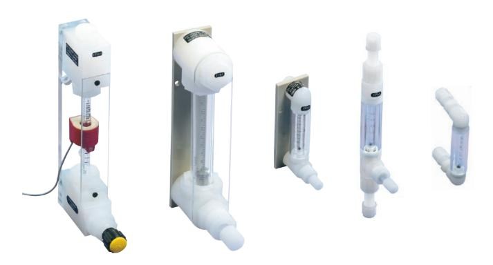
Series 4 flow meters: for demanding flow measurement tasks; these flow meters utilise the float principle and, due to their technical properties, are suitable for precise measurements of gases and aggressive media. Made of Duran® glass and materials such as PP, PVDF, PFA or PTFE, these flow meters are well-suited and highly reliable for a range of applications.
