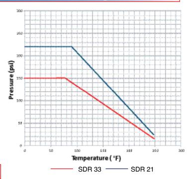
Standard dimensional ratio provides a consistent pressure rating across the entire size range. Super Proline® is offered in two thickness ratios: SDR 33 (150psi) and SDR 21 (230psi). Substantial cost savings can be realized by supplying SDR 33 material starting at Asahi's industry-leading smallest diameter of 90mm. For systems requiring only 150psi, SDR 33 piping and fittings use 35 percent less material than SDR 21.
