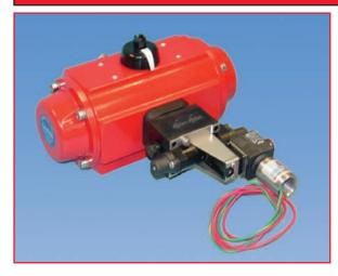
The solenoid valve used for our pneumatic actuators is a four-way, on/off, electrically controlled valve. An electrical signal to the solenoid's coil switches the compressed air supply to the appropriate actuator ports.
