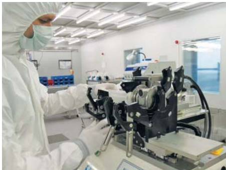
Worker in protective gear using the Asahi SP-110S IR Fusion tool
