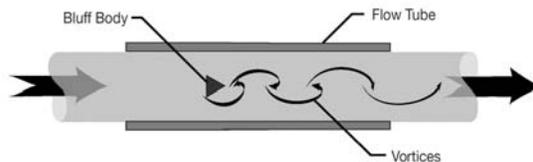
Figure 7.D Vortex Principle
