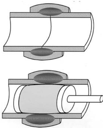
Figure 7.G HPF Fusion without and with internal support balloon
