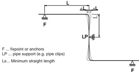
Figure 7.A An Example of one Thermal Expansion Design Options
