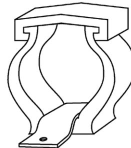
Figure 7.1 Recommended Pipe Hanger Design
