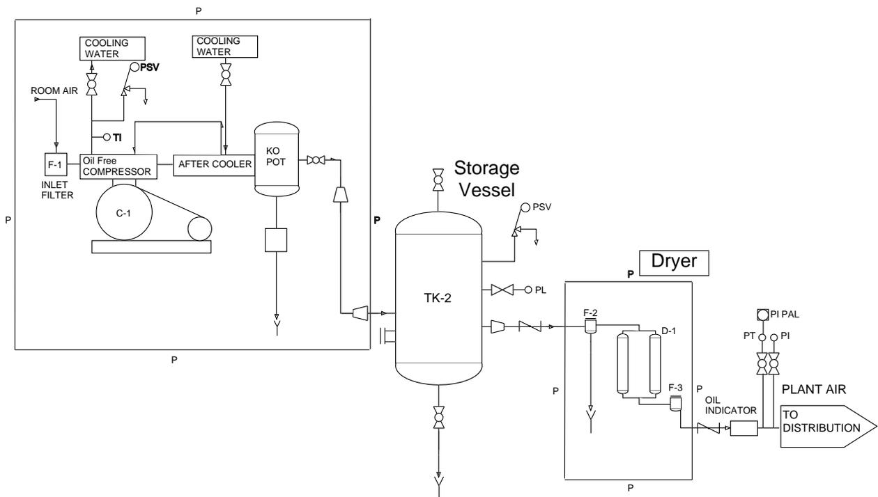
FIGURE 3.E COMPRESSED AIR SYSTEM
