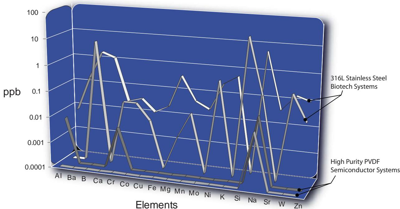
FIGURE 1.A: ION CONTAMINATION COMPARISON BETWEEN FOUR ACTUAL HP INSTALLATIONS. ION CHROMATOGRAPHY MEASUREMENTS TAKEN ON DYNAMIC WATER SAMPLES DEPICT EXPECTED PURITY LEVELS BETWEEN POLYMER AND STAINLESS SYSTEMS.
