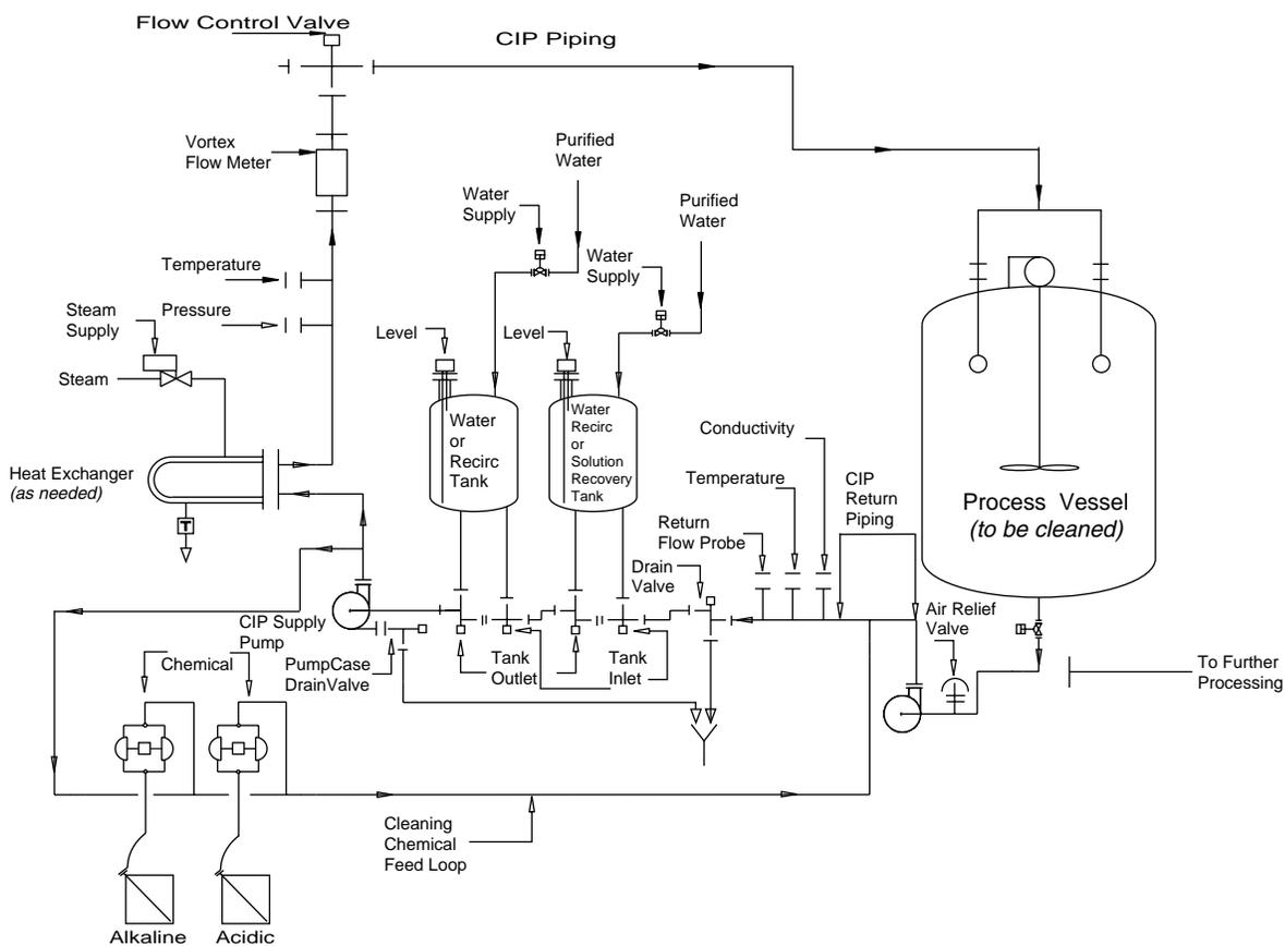
FIGURE 3.D TWO TANK CIP SYSTEM (Note: Either Proline PP or Purad PVDF can be used as piping material depending upon cleaning agent used. Proline PP is excellent for most caustic agents)
