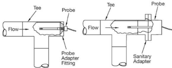
Figure 7.N Instrument probe installation
