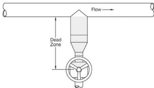
Figure 7.J Improper Dead Leg Design
