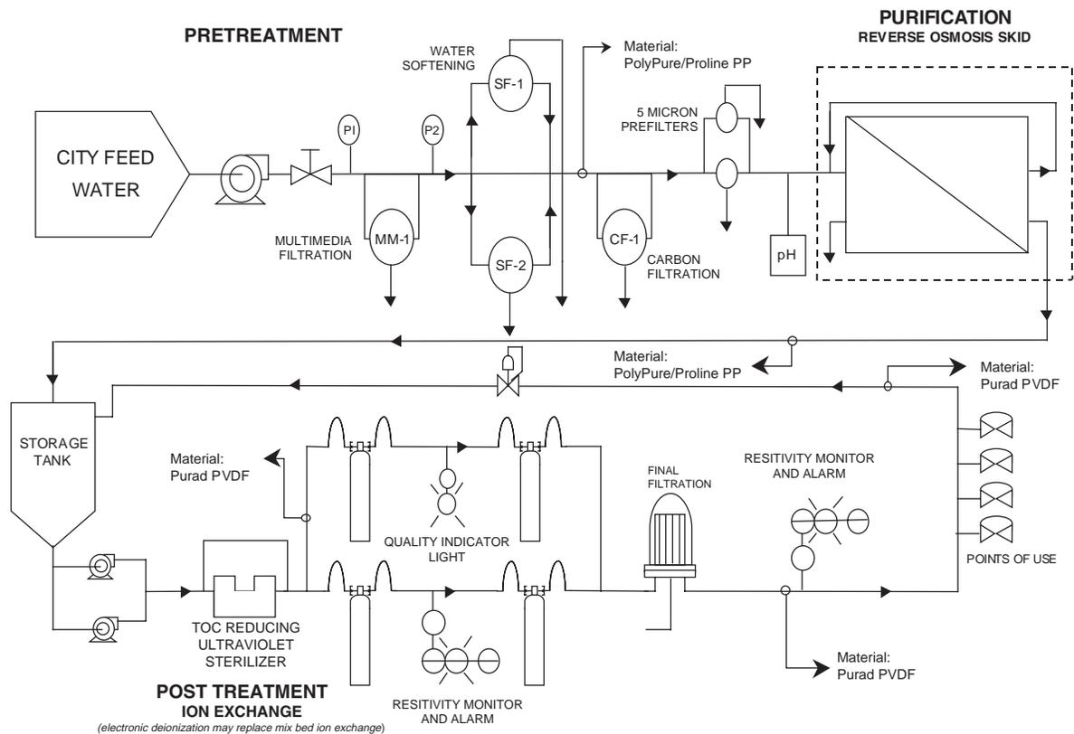
FIGURE 2.A SAMPLE PROCESS PIPING P&ID
