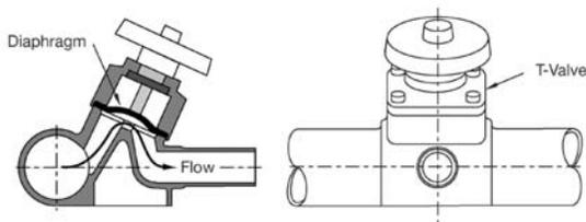
Figure 7.K Molded T-Valve with significantly reduced dead-leg
