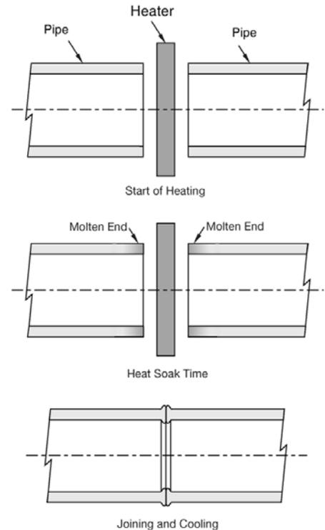
Figure 7.F Steps of IR Non-Contact Fusion
