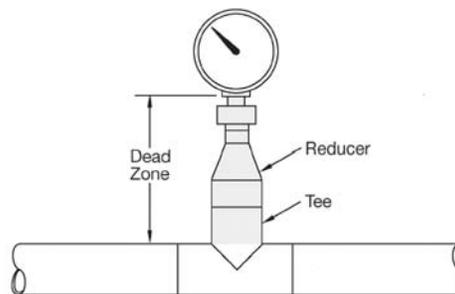
Figure 7.L Dead leg to improper instrument installation
