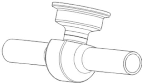
Figure 7.O Sample sanitary instrumentation adapter
